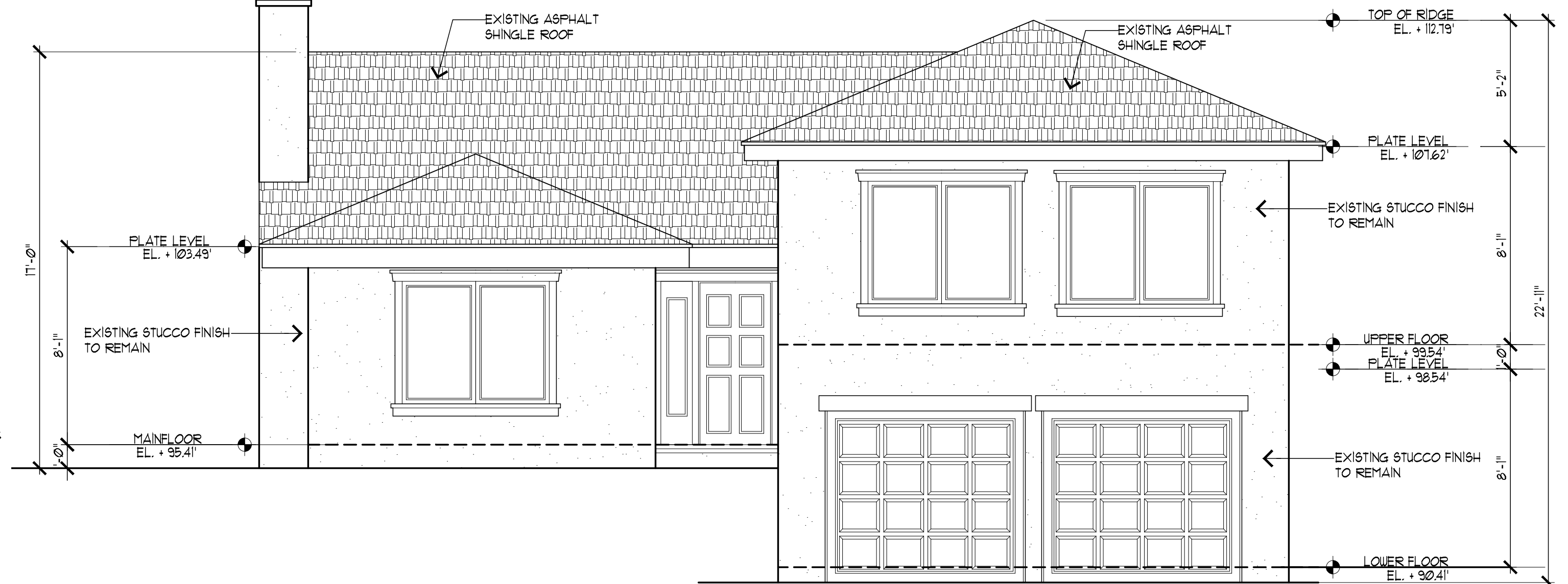
EXISTING FRONT ELEVATION
