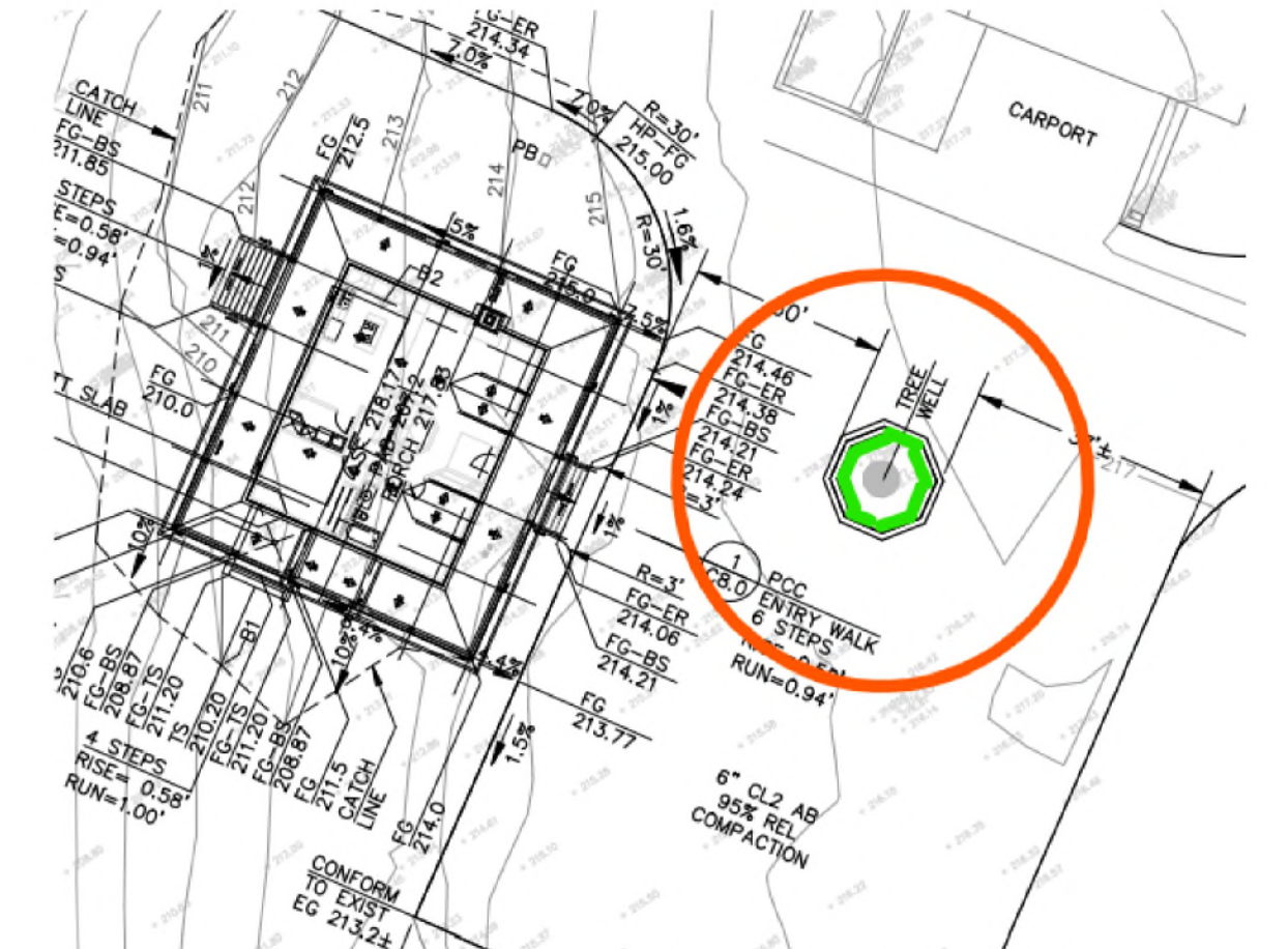
Showing the recommended tree protection fencing locations. Red line indicates tree protection fencing during construction of home. Green line indicates tree protection fencing during construction of the driveway turnaround.
